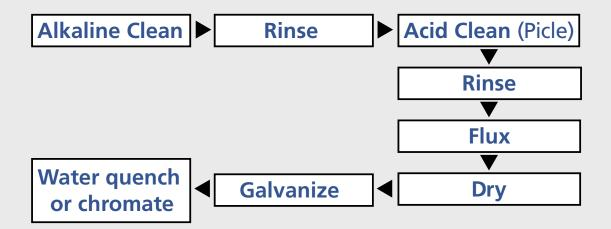
**Surface preparation** for galvanizing typically consists of three steps: caustic cleaning,( to remove organic matter such as dirt, paint, oil and grease.) acid pickling (to remove scale and rust) and fluxing (to prevent oxides from forming prior to galvanizing).
