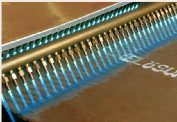
Table 2. Preheating of HARDOX prior to oxy-fuel cutting.
