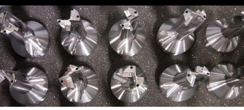
Toolox® is a new steel made by Swedish special steel producer SSAB. Its is delivered with an unique of high mechanical strength and crack resistence. Therefore it is ideal for high performing tooling like U-drills and high speed mills. The high mechanical strength up to 45 HRC takes away the need for heat treatment. Thus shortening lead times and reducing quality problems.
