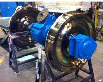
Wheels used in a steel coking plant locomotive. Previoulsy the wheels were made from forged steel which was a well working solution. The disadvantage was the long lead times once the wheels needed to be replaces. Making the wheels out of Toolox® 44 plates solved the problem.
