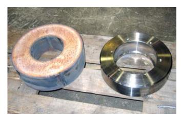
Crane steering wheels in a steel plate rolling mill. The wheels are normally changed every 3–5 years. Previously 35CrNiMo14 (similar to W.Nr.1.6582) machine steel was used. The wheels where induction hardened to a depth of 10 mm. Now Toolox® 44 with no surface treatment is used. Large advantage in manufacturing is achieved since time is saved due to no need of heat treatment. Furthermore, cutting the rings from plate saved machining time and guaranteed a homogeneous small grain structure.
