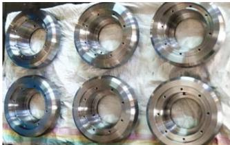
Guide rollers in cement mill stacker/reclaimer. In the previous solution case hardened 42CrMo4 was used. Changing to Toolox® 44 decreased lead time with 10 days due to no need to send the rollers for heat treatment. A much better surface finish with Toolox® gives better resistance to adhesive wear.
