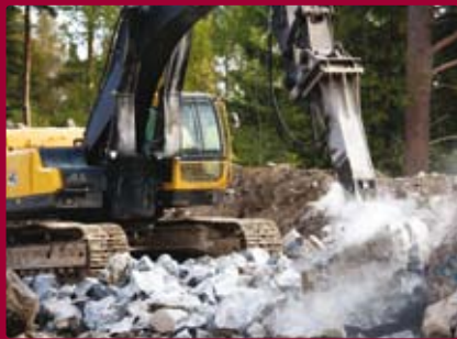
HYDRAULIC HAMMER Hardox 400/450 in the housing of the hydraulic hammer exposed to wear from rocks.
