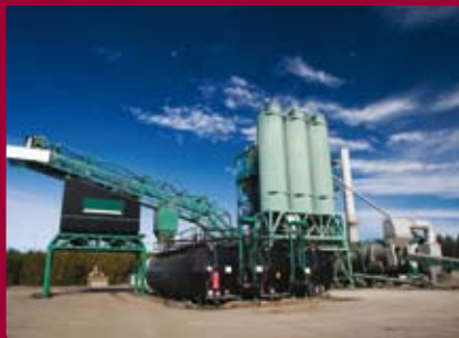
ASPHALT PLANT Hardox 450/500/550 as liner plates and in gravel chutes. Hardox 450/500 in the wings of the drum. Hardox 450/500 in the transport container from the drum to the truck delivery shaft.
