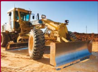
MOTOR GRADER Hardox 450/500/550 in the blades of the motor grader.
