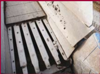
CHUTE In the chute that leads into the crusher Hardox 500/550/600 is the obvious choice in the tough environment.
